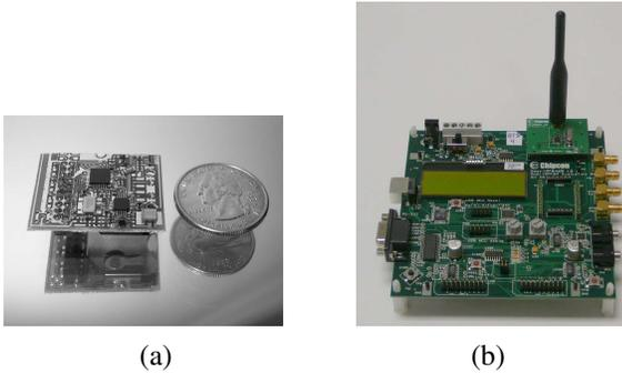
**Figure 2.** (a) PIP. (b) Base-station: Texas Instruments CC1100/CC1150-868/915 MHz Development Kit
