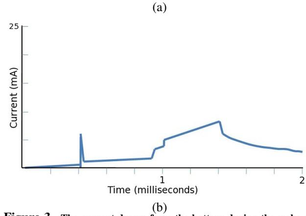
**Figure 3.** The current drawn from the battery during the wake up and transmission part of the duty cycle, before and after the addition of a 100 microfarad chip capacitor.
